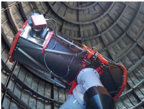
SkyVision 400 telescope under dome in autonomous control
